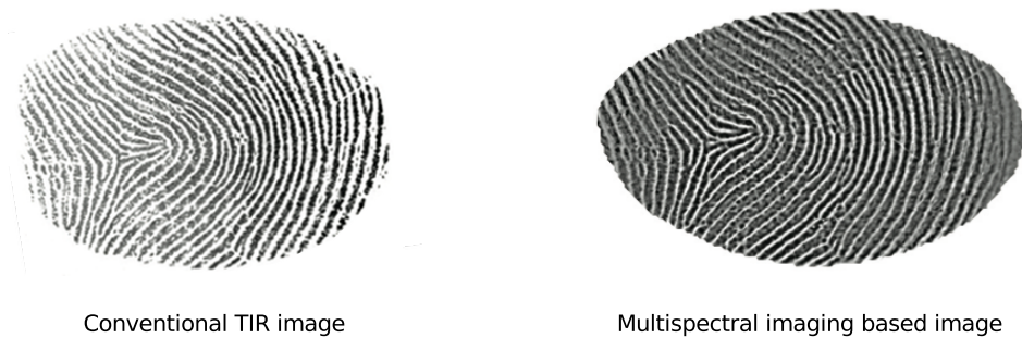
Figure 2.7: Example for application field of biometrics. A conventional TIR image is compared to a composed multispectral fingerprint image of one finger. As can be seen, fine structures are visible throughout the multispectral image. The images were overtaken from [RNB08].
