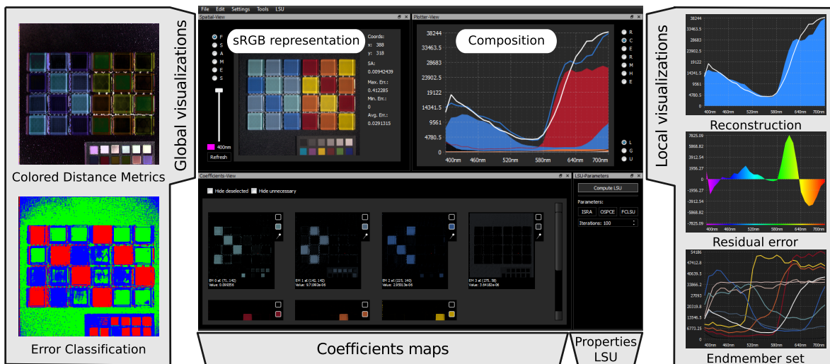
Figure 5.18: Overview of the graphical user interface, that focuses on several linked views, achieved coefficients maps, global spectral error views and per-pixel views for detailed local investigations.
