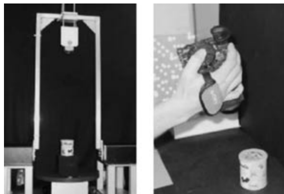
Fig. 1. Left: turntable with camera arm. Right: handheld camera.
