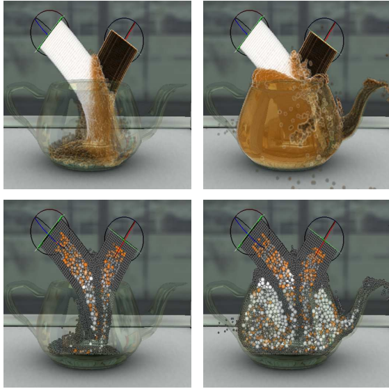
Figure 3: Mixing of coffee and cream in an Utah Teapot. Blend-sets (bottom) are used to dynamically adapt to the convective and the diffusive flux (top), shown for t=2 and t=6 .
