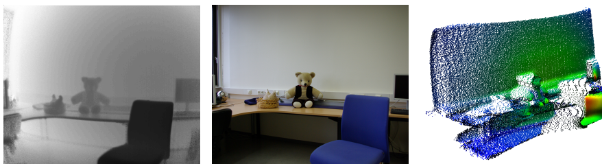
Figure 1: Example of a depth image. Left: The depth map, where darker means nearer. Middle: A color picture taken with a normal camera from the same position. Right: A Point cloud computed from the depth map, shown from a different perspective.
