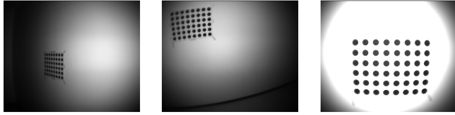
Figure 9: Example pictures of the lens calibration. In total, 41 such pictures are used for the calibration.
