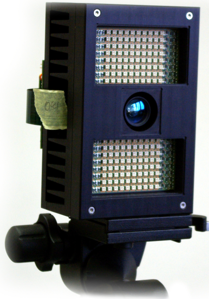
Figure 7: The PMD DigiCam prototype. Above and under the lens are two powerful LED-arrays which illuminate the scene. The backside consists mainly of the cooler.
