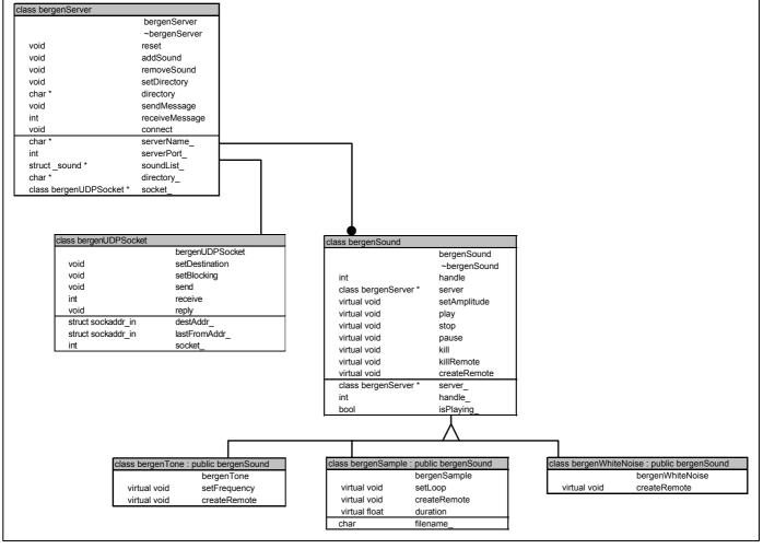
Figure 8: OMT Diagram client components
