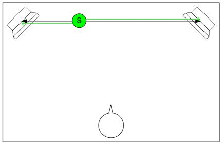
Figure 18: Stereophonic sound positioning using two loudspeakers
