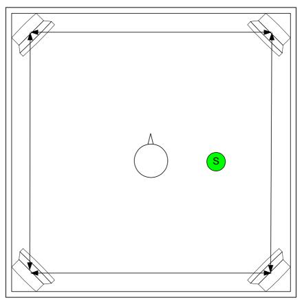
Figure 39 : Sound reproduction with listener in hotspot using 4 channels with 50% amplitude both of the right speakers
