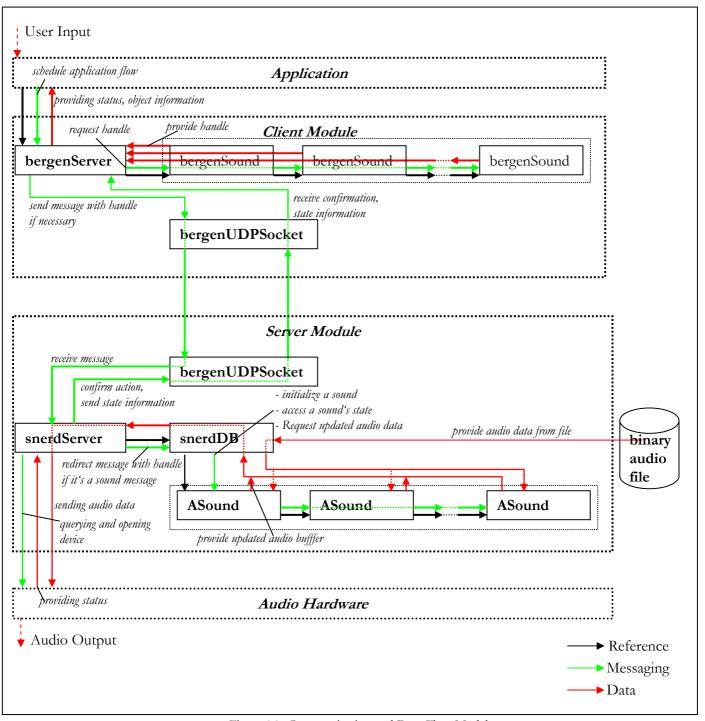
Figure 16: Communication and Data Flow Model
