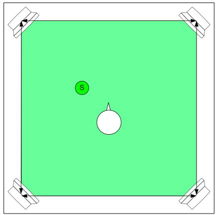
Figure 19: Sound positioning using four loudspeakers
