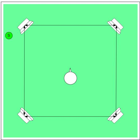
Figure 20: Sound positioning using four loudspeakers with additional overall amplitude adjustment
