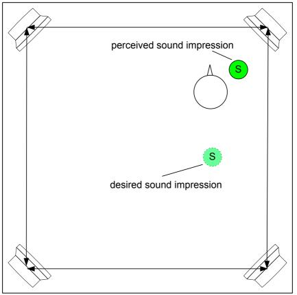
Figure 40 : Failure in sound reproduction through physical listener movement
