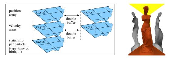
Fig. 4. Data storage concept for particle systems (left) and two depth-maps as parts of a complex boundary representation of a statue (right).
