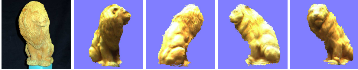
Figure 6. RGBz lightfield example from [32] using a ToF-sensor . A PMD Vision 19k cameras has been used. The artefacts result from the inaccurate depth information at the object boundaries.
