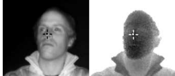
Figure 5. Example nose-detection results shown on ToF-intensity (left) and ToF-range image (right); detection error rate is 0,03 [4]. A MESA SR3000 cameras has been used.
