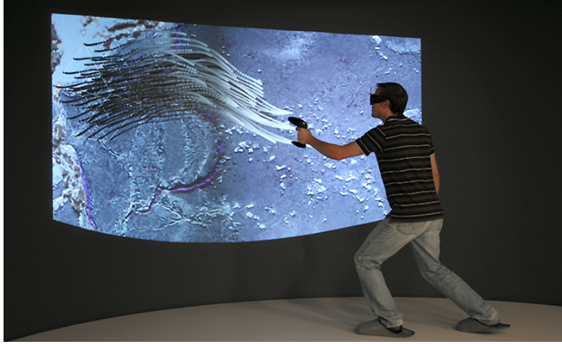
Figure 4.22: Flow visualization of a typhoon in the VR laboratory of the University of Siegen, including user interaction using tracking devices. The glasses are tracked in order to render the correct point of view. The so-called flystick controls the placement, orientation and size of the emitter box from which streak lines originate.
