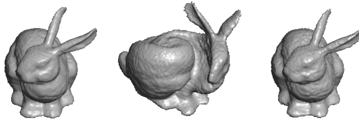
Figure 3.14: The "Stanford bunny" in a deforming vortex flow: initial, after 40 advections, after backward advection. 131,072 particles, 96^3 grid, 40.47 FPS.
