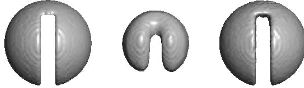
Figure 3.13: 360^\circ rotation of Zalesak's sphere (100 advections): initial, LS, and PLS. 524,288 particles, 128^3 grid, 14.74 FPS.
