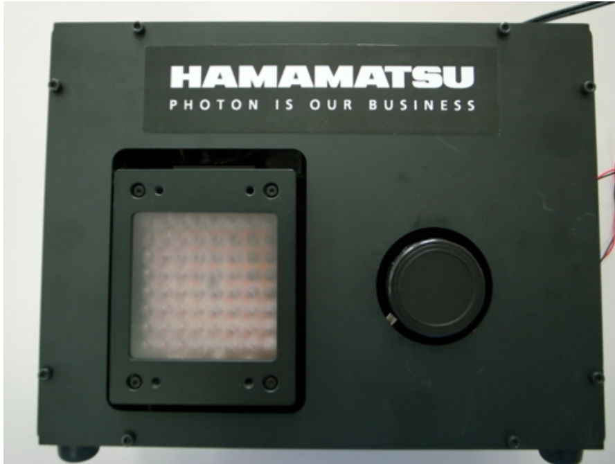
Figure 8: The used camera system with illumination unit (left) and the lens (covered, right). [Ham14]
