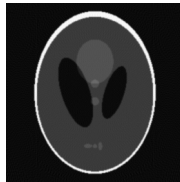
Figure: Filtered backprojection with Shepp-Logan filter (angle increment: 10 degrees (left), 1 degree (middle), difference image of original Shepp-Logan phantom and reconstruction result with 1 degree increment (right))
