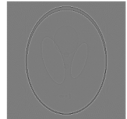
Figure: Filtered backprojection with Shepp-Logan filter (angle increment: 10 degrees (left), 1 degree (middle), difference image of original Shepp-Logan phantom and reconstruction result with 1 degree increment (right))
