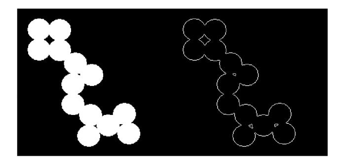
Erosion with respect to the structuring element in shape of line (original image in right):
