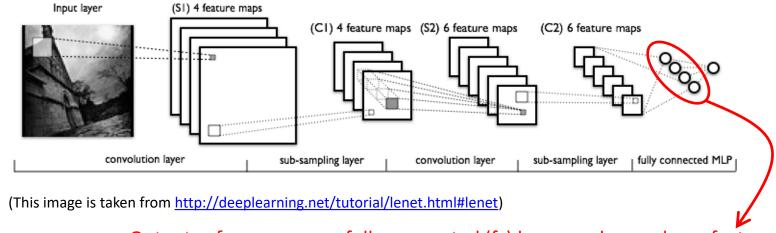
Outputs of neurons on a fully-connected (fc) layer can be used as a feature
