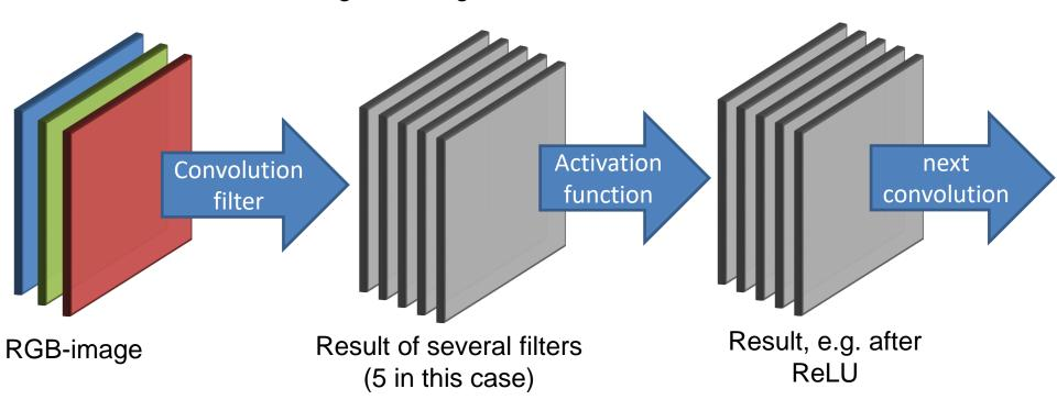
The number of filters determines the number of channels in the next layer!
